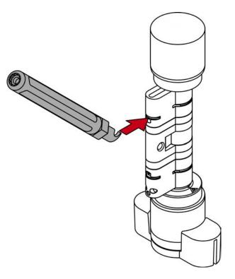
3. Lever the clamp out of the profile cylinder by moving the extractor to the centre of the cylinder.
