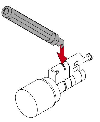
7. Lever the second clamp out of the profile cylinder by positioning the lifter in the centre of the cylinder.
