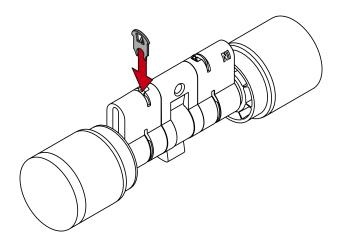
└→ Cam on the SI Digital Cylinder AX has been replaced.
