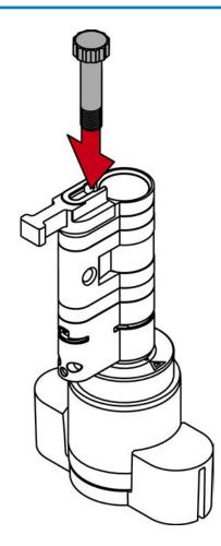
11. Reassemble the two cylinder halves.
