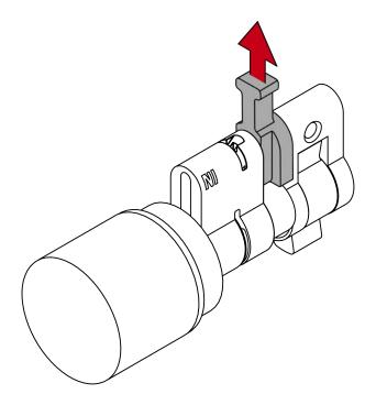
16. Push the halves together completely.
