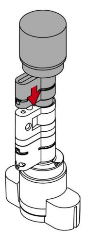
14. Refit the clip into the slot of the profile cylinder with the lug facing the fastening screw.
