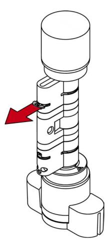
5. Disassemble the two cylinder halves.
