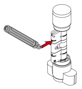
3. Lever the clamp out of the profile cylinder by positioning the lifter in the centre of the cylinder.
