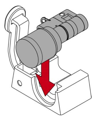
12. Refit the clip into the slot of the profile cylinder with the lug facing the fastening screw.
