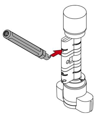
3. Lever the clamp out of the profile cylinder by moving the extractor to the centre of the cylinder.
