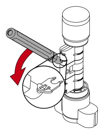
4. Pull the clamp out of the profile cylinder completely.
