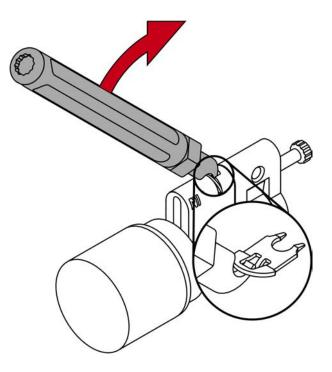
8. Pull the second clamp completely out of the profile cylinder.
