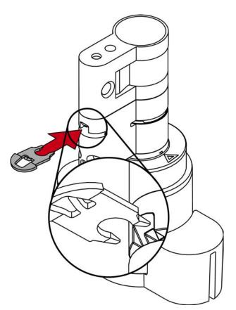
13. Insert the cylinder into the clamping block so that the profile cylinder and the thumb-turn lie flush in the recesses.
