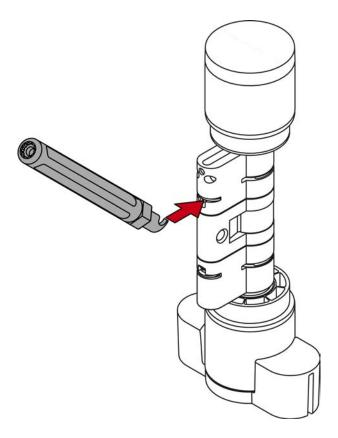
3. Lever the clamp out of the profile cylinder by moving the extractor to the centre of the cylinder.
