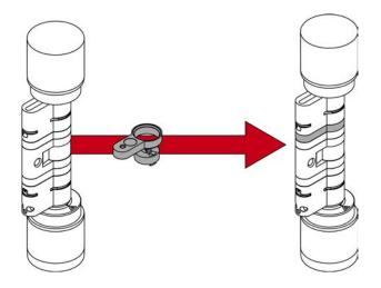
The core extension and profile extension must be the same length. You also need an extension bolt for the desired length.
