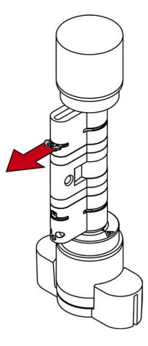
5. Disassemble the two cylinder halves.
