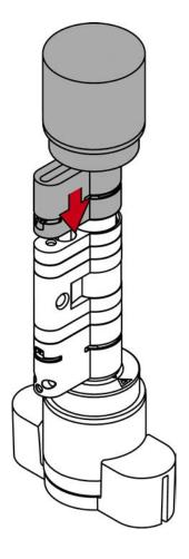
14. Place the clip back into the slot of the profile cylinder with its lug facing the fastening screw and press the clamp with your thumb so that it can no longer fall out.
