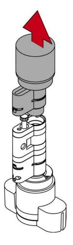
6. Unscrew the bolt with the extractor.
