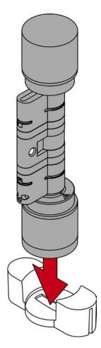
2. Hook the tip of the extractor into the clamp.
