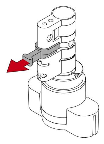
11. Push the cylinder parts together completely.
