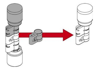
You can use a special centre piece to assemble a half cylinder from an AX comfort cylinder or a freely rotating cylinder.
