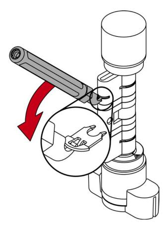
4. Pull the clamp completely out of the profile cylinder.
